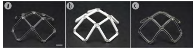
Figure 9: The pipes are replaced with soft materials such as (a) acrylic; (b) PLA; (c) rubber. (Scale bar: 10 mm)
