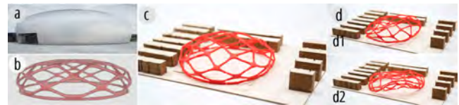
Figure 14: Architecture design enabled by FlexTruss: (b) an architect can input a stadium (adapted from [36]) to the design platform, and (b) nodes will be generated; (c) the stadium as fabricated; (d) the architect can manipulate the FlexTruss stadium to illustrate their design to the audience.
