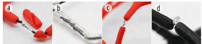
Figure 10: Knotting method: (a) a split node can hide the knot easily; (b) pipes can be cut for hiding the knot; (c) coiling two ends of the wire together for closing the loop; (d) a TPU knot.
