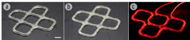
Figure 7: The materials of threading wire: (a) PVC coated wire; (b) elastic rope; (c) optical fiber. (Scale bar: 10 mm)
