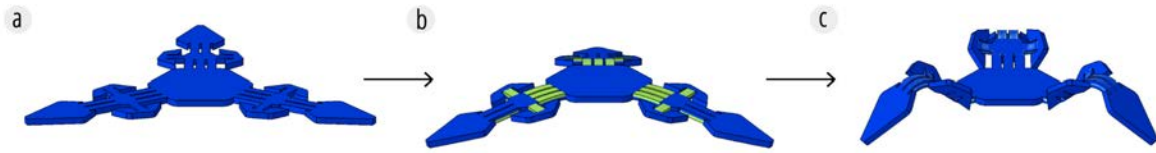
Fig. 7. The simulation result of the sequential transformation: (a) the initial geometry; (b) the intermediate transformation under the influence of body force creeping; (c) the final transformation after residual stress releasing.
